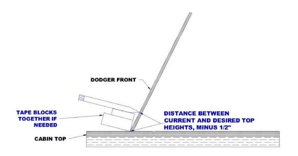
Trim the front with a jigsaw. Position the dodger back on the boat. Mark and re-trim the dodger as needed for the best fit. Small adjustments can be made by block or machine sanding when it's difficult to get a straight edge with the saw.
